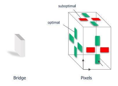
Optimal pixel orientation shown in green, and suboptimal in red, relative to the energizing bridge antenna. In the drawing, the antenna's dual linear polarizations are aligned with the y axis and z axis.
